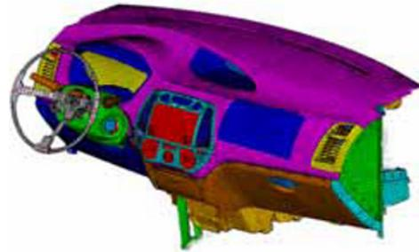
Fig. 6. Finite-element model of cockpit module.
