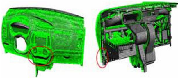
Fig. 10. Result of analysis (permanent deformation).
