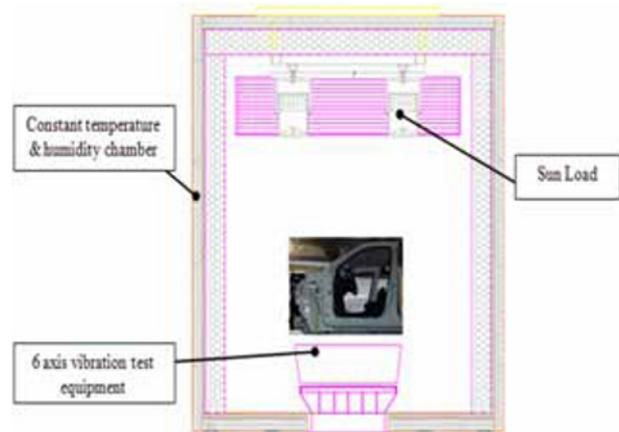
Fig. 2. Key-life test device diagram.
