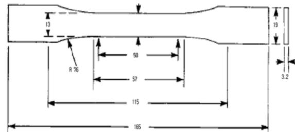
Fig. 4. ASTM D638 Type 1 specimen.
