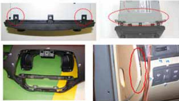
Fig. 11. Result of key-life test (permanent deformation).
