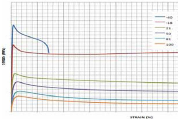
Fig. 5. Results of tension test at each temperature.
