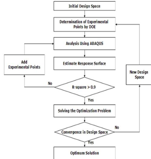
Fig. 12. Flowchart of methodology for optimal design of mount positions.
